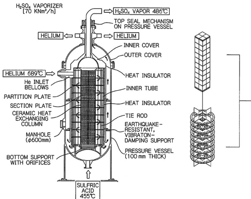
Fig. 3. Schematic of ceramic heat exchanger for use in a high-pressure, high-temperature  $\text{H}_2\text{SO}_4$  vaporizer unit [14].
