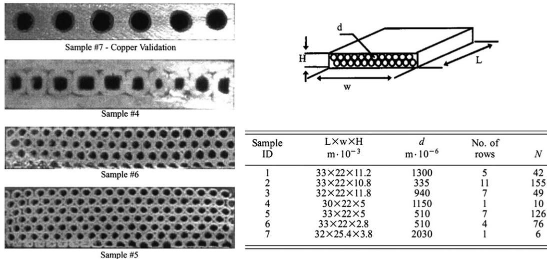
Fig. 10. Photographs and schematic of representative SiC heat sink samples [26].
