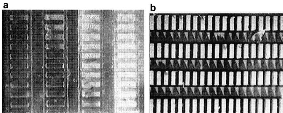
Fig. 5. (a) Polymer “lost mold” and (b) fully-dense silicon nitride sintered part [17].
