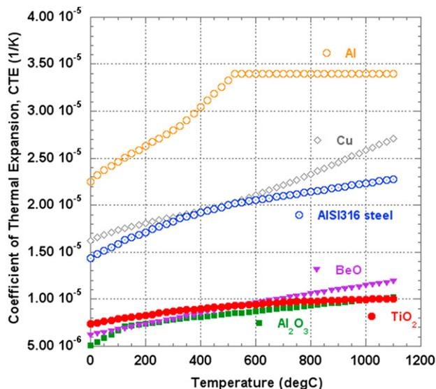
Fig. 13. The difference in linear thermal expansion between metals and ceramics can be significant.
