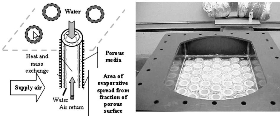
Fig. 4. Ceramic pipe heat exchanger utilizing both heat and mass transfer [15].
