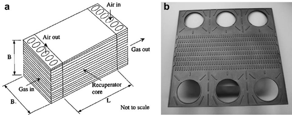
Fig. 6. (a) Schematic of the heat exchanger body showing the flow directions and (b) a sintered SiC process gas plate [3].
