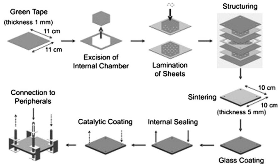
Fig. 15. Manufacturing process for the construction of a ceramic plate heat exchanger from green tape [32].
