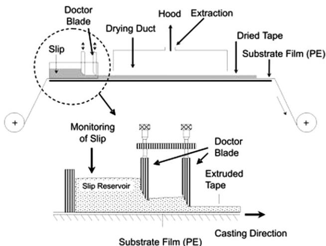
Fig. 16. The so-called doctor blade process for the production of green tape [32].
