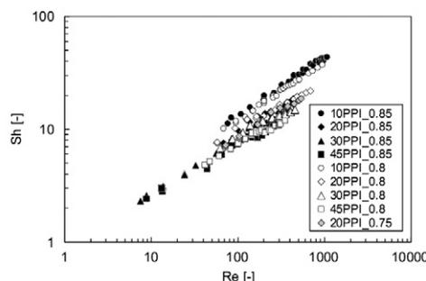
**Fig. 18.** Experimental Sherwood number data as a function of the Reynolds number for nine different alumina foam samples [57].
