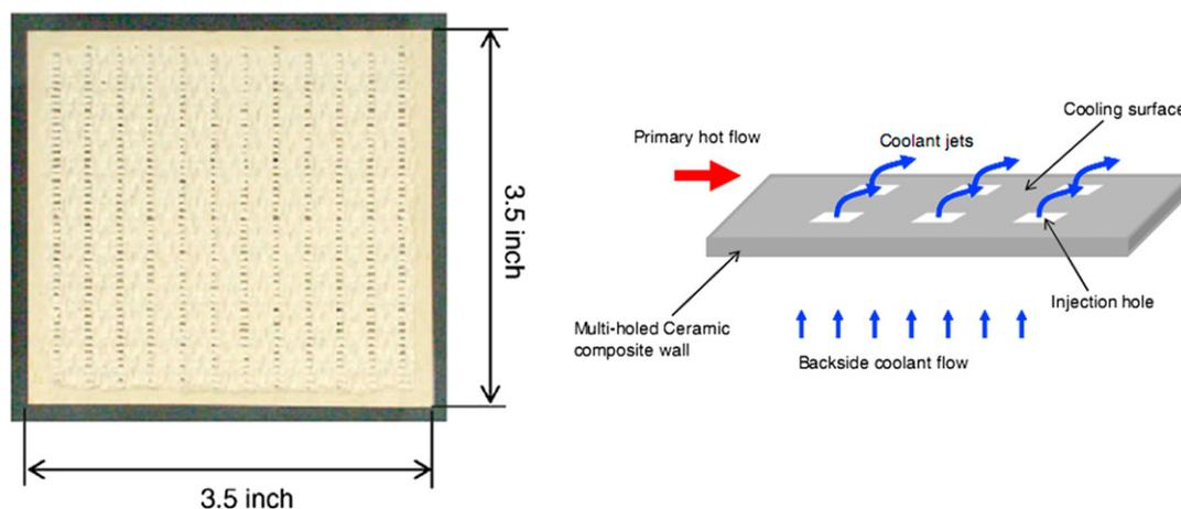
Fig. 9. Integrally-woven SiC/SiC ceramic matrix composite materials for gas turbine applications [22].
