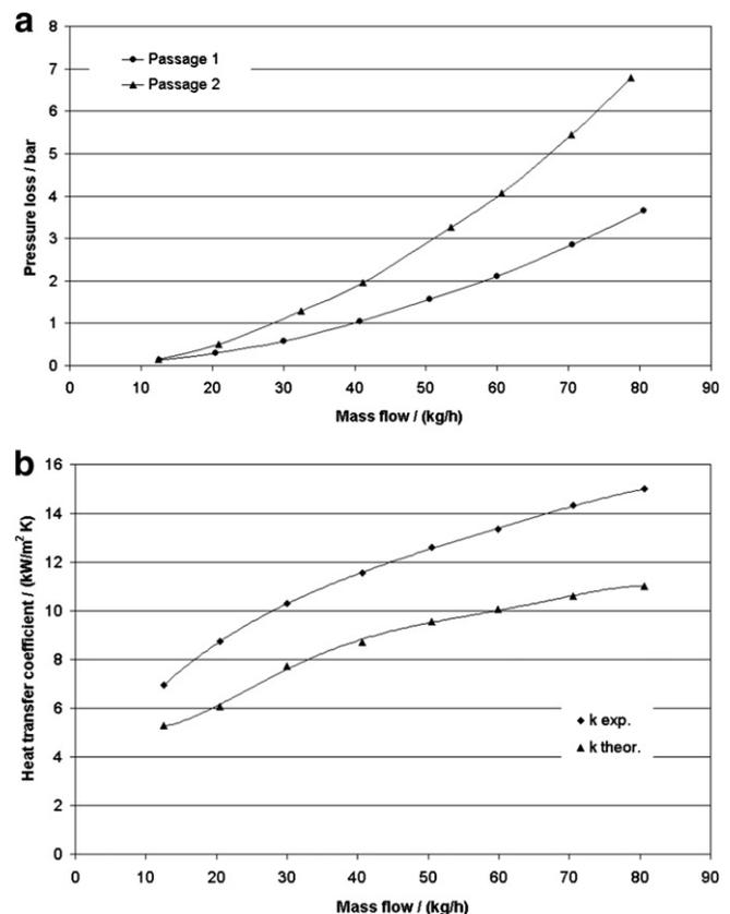
**Fig. 2.** (a) Pressure drop and (b) heat transfer coefficient data for various water mass flow rates (1-cold stream, 2-warm stream) [7].
