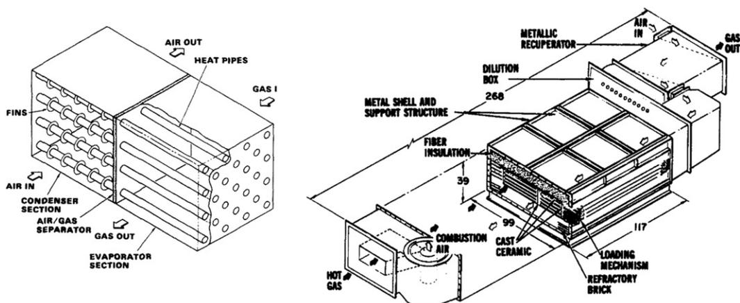
Fig. 7. Schematic of a ceramic heat pipe recuperator [18].
