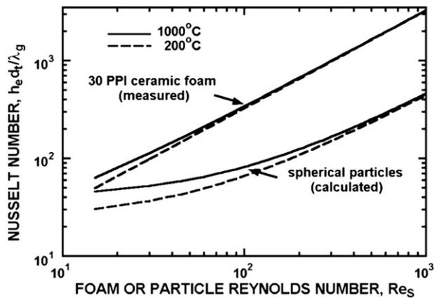
Fig. 19. Heat transfer comparison between equivalent 30-PPI  $\alpha$ - $\text{Al}_2\text{O}_3$  foam and particle beds [54].
