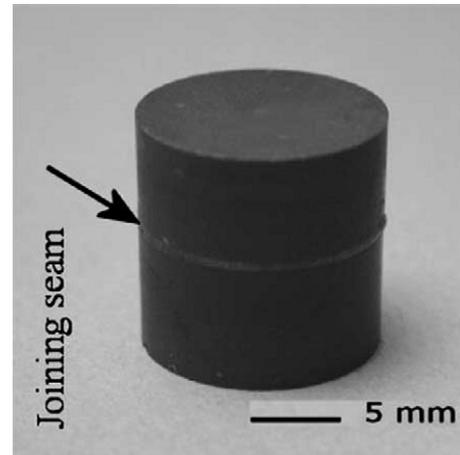
Fig. 14. Laser bonded hollow SiC capsule showing the applicability of the laser induced soldering technique [31].
