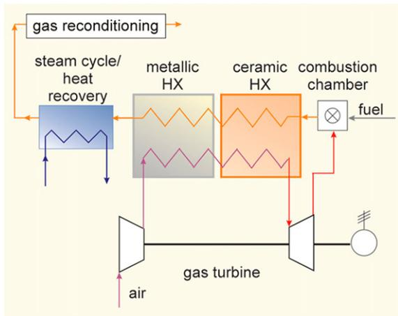
Fig. 8. Combined cycle gas turbine power plant with a high temperature ceramic heat exchanger [3].
