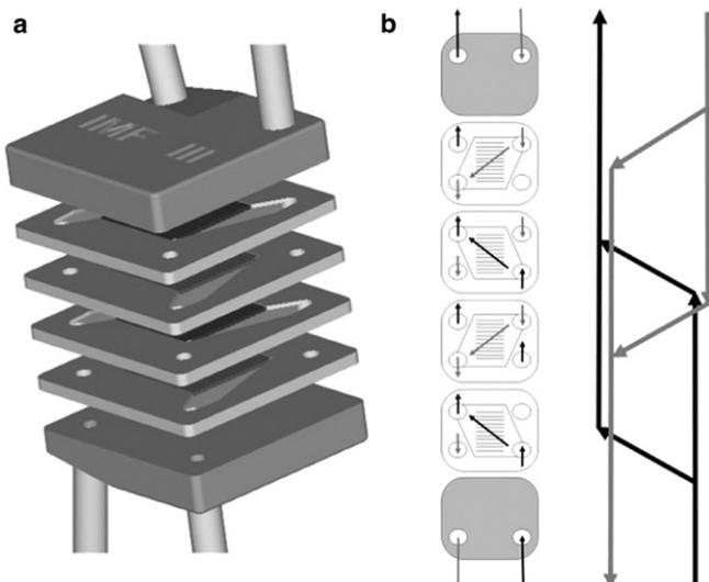
**Fig. 1.** Ceramic micro heat exchanger construction and cross-flow arrangement [7].
