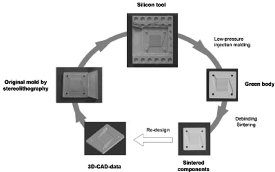
Fig. 17. Rapid prototyping process for the manufacture of ceramic heat exchangers [7].
