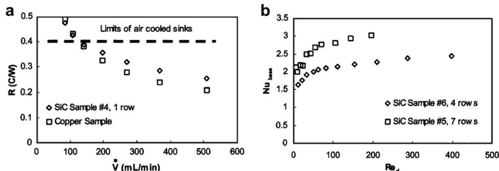
Fig. 11. (a) The thermal resistance of water-cooled heat sinks is significantly lower than air-cooled sinks for modest flow rates, and (b) the Nusselt number based on base area was observed to increase as the number of rows increased [26].
