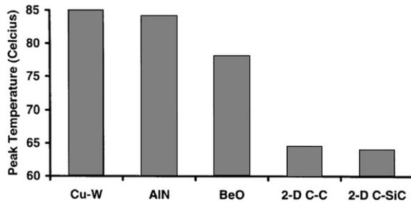
Fig. 12. Thermal Spreader Results [27,28].
